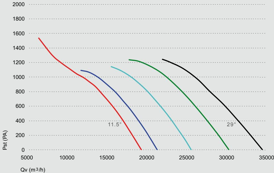
DN63V 2 pole long casing measured with inlet bell-mouth in installation type A according to ISO 5801
